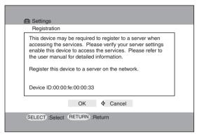
5 Press the direction arrow buttons to highlight **OK**, then press the **SELECT** button.
